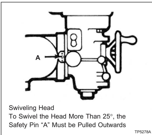
Figure 1.2 - Positioning Head
