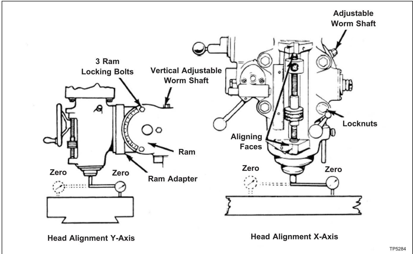
Figure 1.9 - Head Alignment for Y- and X-Axis
