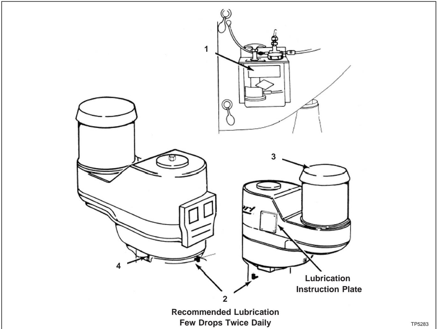
Figure 1.8 - Lubrication Requirements
