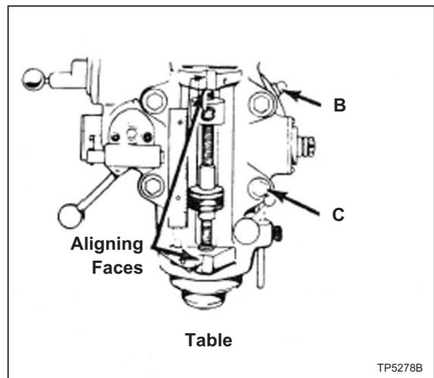
Figure 1.3 - Positioning Head
