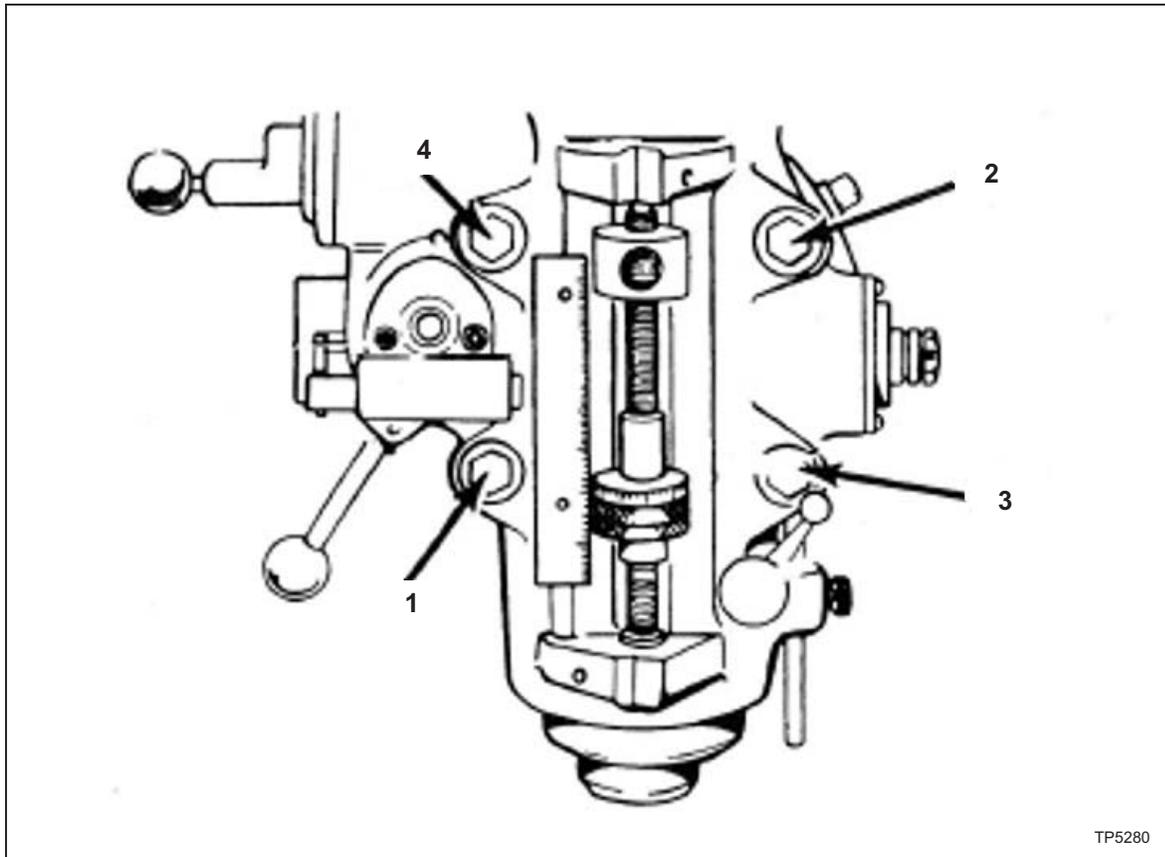
Figure 1.5 - Tightening Sequence
