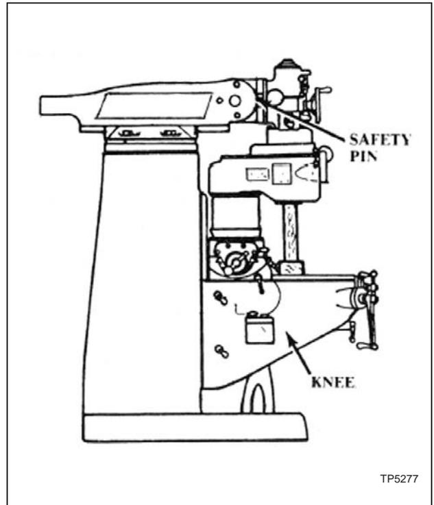
Figure 1.1 - Milling Machine
