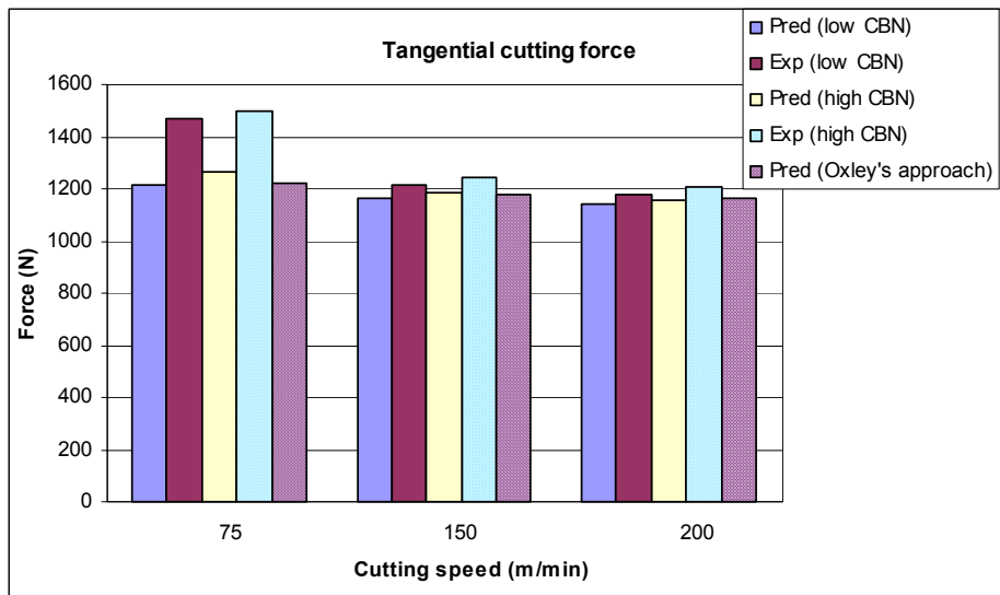
(b). Tangential cutting force with cutting speed 75,150, and 200m/min
