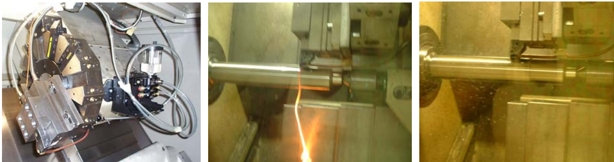
Figure 1 Minimum quantity lubrication applicator fitted to a horizontal lathe (on left). Dry machining (on center). Minimum quantity lubrication machining (on right).
